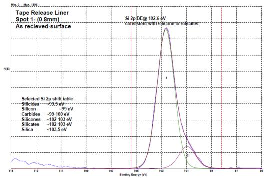
This is a high resolution scan which scans over a smaller range of binding energies and enables the detection of slight shifts in binding energies that normally represent different chemical states. Ex: A high-resolution scan of the silicon peak confirms silicones and a minor amount of another silicon state.
