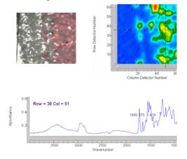
A spectrum taken from the data set at the location of the cross hairs is also shown. This represents a 5.5 micron area on the sample. Each spectrum has a similar signal to noise ratio as this one and the
