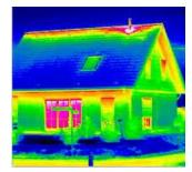
type of thermal image that is taken to determine heat leakage from a home during an energy audit.
