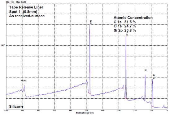
This is a typical "survey" or wide range scan. Scanning from 0-1100 eV it detects an element on the surface that is >0.1 At %. Ex: The surface of a Tape release liner has a silicone coating based on the 2:1:1 ratio of C:O:Si.
