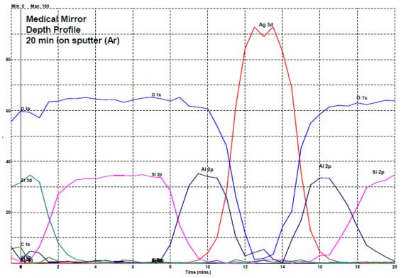
A depth profile can help one understand how the material changes as a function. Different materials have a different sputter rates so only approximate thickness can be assumed without standards. Ex: Above after a 20 minute profile the thin films of a medical mirror are zirconium oxide, silicon dioxide, aluminum oxide, silver, aluminum oxide and silicon dioxide.
