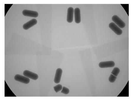
Inspection of pharmaceutical tablets for damage during manufacturing, while still sealed in their sterile foil pouches.
