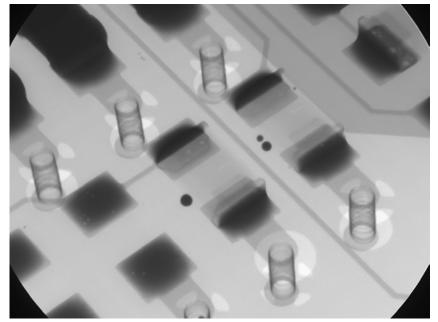
Angle view of printed circuit board with surface mount components. Note small, spherical solder balls loose inside the sample (center of view), which can possibly lead to electrical shorts if loose inside the package.
