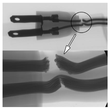
Failed conductor in a household appliance. Note the melting of the individual conductors caused by arcing (near the tip of the white arrow).
