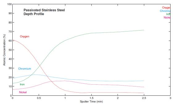
Depth profile (measurement of concentration versus depth into the sample) of Stainless Steel
